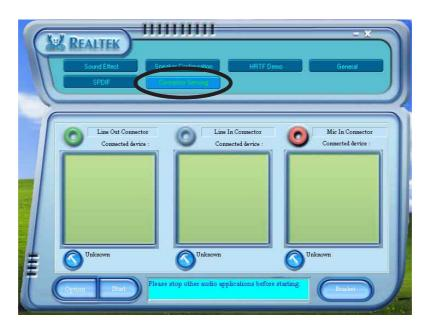
5. When finished, the utility prompts the Realtek® EZ-connection dialog box showing your current audio connections. The text at the bottom of the box explains your audio connection status. An *X mark* denotes an incorrect connection.
